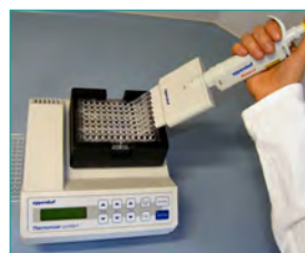
6. Washing (removal of unbound components, 2x1min)
