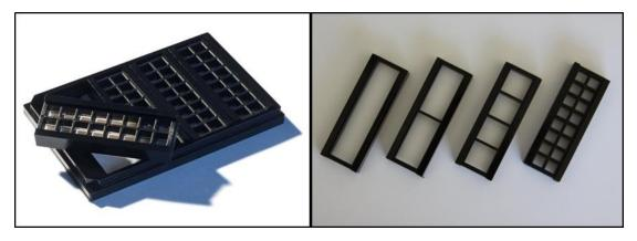
**Figure 8.** ProPlate chambers enable active mixing of sample during hybridization. The chambers attach to slides for hybridization and are removed for imaging.
