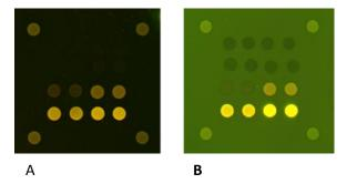
**Figure 6.** Effects of proper blocking on ONCYTE<sup>®</sup> film slides. (A) Slide blocked with Grace Bio-Labs Super G Protein Array Blocking Buffer for 1 hour prior to assay. (B) Slide not blocked (soaked in PBS for 1 hour) prior to assay.
