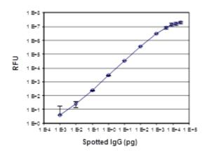
**Figure 3.** Dynamic range of protein binding for ONCYTE® AVID film slides spans over 7 orders of magnitude with a linear range of 6 orders of magnitude ( $r^2 =$ 0.999). Data are normalized, backgroundsubtracted fluorescence intensities collected at 532 nm from spotted goat lgG-Cy3. Data presented are the mean ± standard deviation for N = 4 slides (20 spot replicates per spotting concentration per slide).
