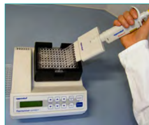
6. Washing (removal of unbound components, 2x1 min)
