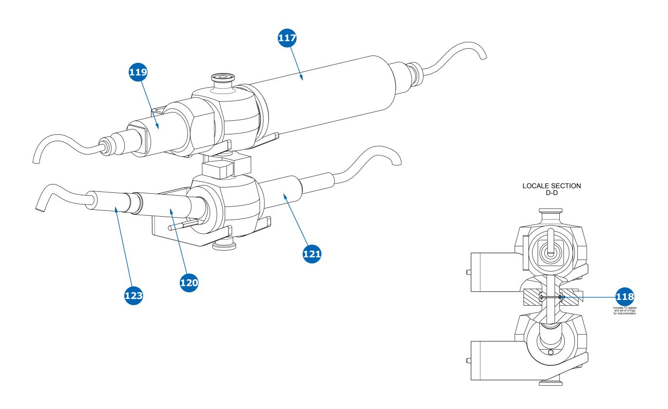
XMO1/2 & XMO3 Multi-Use Pre-Column Instrumentation (pH/Conductivity)
