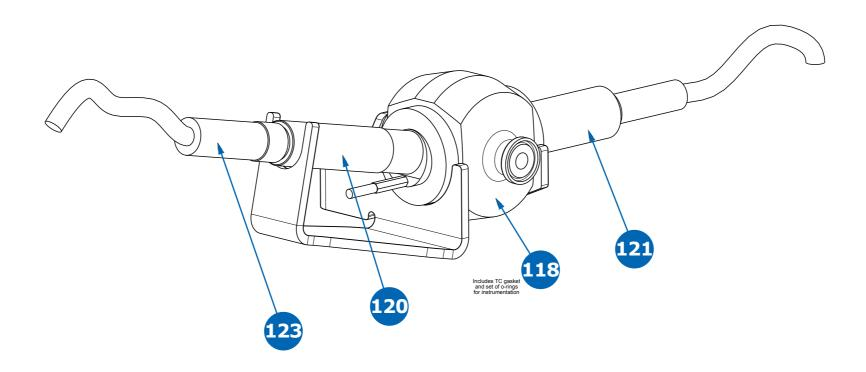
XMO1/2 & XMO3 Single-Use Post-Column Instrumentation (pH/UV/Conductivity)
