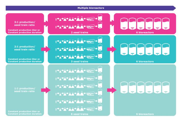
**Figure 3.** The study also considered multiple bioreactor scenarios; constant production titer versus constant duration were evaluated using a model of six bioreactors. In addition, the process modeling included different production to seed train ratios as another variable. For a 3:1 ratio, one seed train was used for every three bioreactors; for the 2:1 ratio, one seed train was used for every two bioreactors. For the 1:1 ratio, every bioreactor had a dedicated seed train.
