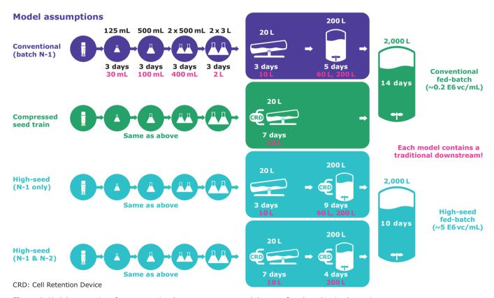
Figure 1. Model assumptions for a conventional upstream process and three perfused seed train alternatives.
