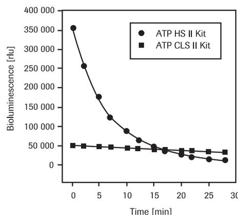
**Fig. 1:** Kinetics of light generation of the ATP Bioluminescence Assay Kit HS II and the ATP Bioluminescence Assay Kit CLS II. 10 pmol ATP in a volume of 50 µl was assayed with 50 µl luciferase reagent in a black microtiter plate.
