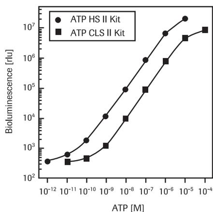
**Fig. 2:** Sensitivity range of the ATP Bioluminescence Assay Kit HS II and the ATP Bioluminescence Assay Kit CLS II. ATP dilutions in a volume of 50  $\mu$ l were assayed with 50  $\mu$ l luciferase reagent in a black microtiter plate on a Berthold LB-96-P luminometer. The light signal was integrated for 10 s after a delay of 1 s.
