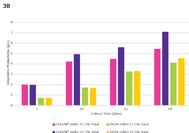
Figure 3. The impact of feeding schedules with Cellvento ® ModiFeed Prime COMP using different cell lines. Viable cell density (3A solid lines), viability (3A dashed lines), and volumetric productivity (3B) during a 14 day fed-batch process for CHOZN ® mAb1 cultured in Cellvento ® 4CHO COMP and DG44 mAb3 cultured in EX-CELL ® Advanced CHO fed-batch medium.
