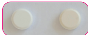
Figure 12. Color of tablets manufactured using ODT excipient system E (right tablet) vs. Parateck® ODT tablet (ODT excipient system A) after 26 weeks storage at 40 °C/75% r.H.
