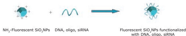
Figure 1. Electrostatic adsorption of DNA molecules on amine-modified fluorescent Silica NPs.
