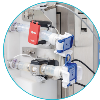
Flexware® assembly with CPC® AseptiQuik® connectors enabling closed processing
