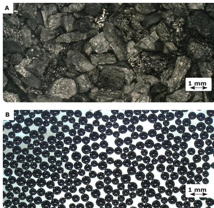
Figure 1. Optical micrographs of A) Granular Activated Charcoal and B) Carboxen® Synthetic Carbon.
