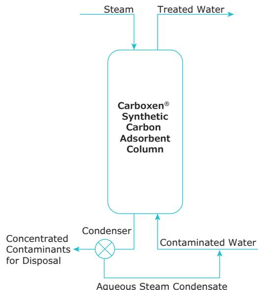
**Figure 3.** Carboxen® Synthetic Carbon closed loop adsorption/regeneration system for water purification
