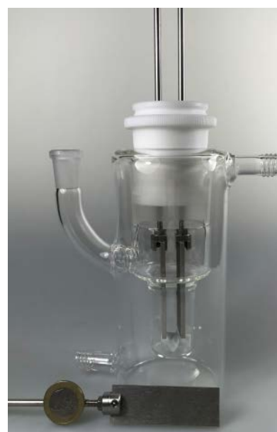
Figure 6. Beaker-Type Glass Cells for Batch-Type Electrosynthesis (25 mL) with Temperature-Control Jacket. Front: Electrode Holder with Mounted Electrode and a 1 Euro Coin for Size Comparison (Diameter 23.25 mm / 0.915 inch).
