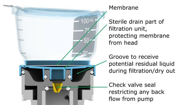
**Figure 1:** The Milliflex Oasis<sup>®</sup> pump head with a filtration device: pump head (gray), filtration device (blue), and the check-valve seal (yellow).
