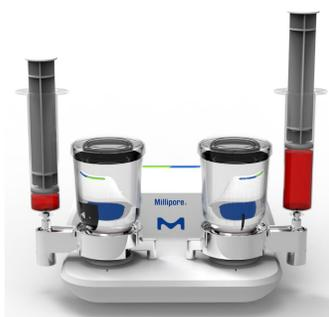
**Figure 2:** Decontamination accessory installed on each head of a Milliflex Oasis<sup>®</sup> pump. 50 mL of the disinfectant is kept in contact with the fluid path for 15 minutes and rinsed with 250 mL of sterile water.
