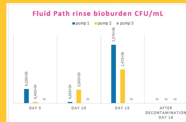
**Figure 3** – graph of pump drain rinsing bioburden level in CFU/mL.
