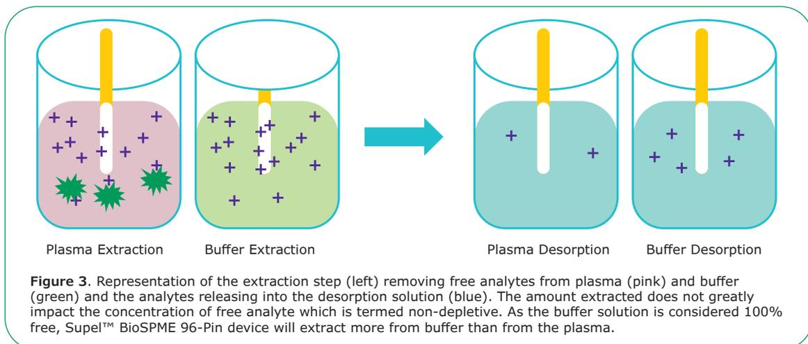
**Figure 3.** Representation of the extraction step (left) removing free analytes from plasma (pink) and buffer (green) and the analytes releasing into the desorption solution (blue). The amount extracted does not greatly impact the concentration of free analyte which is termed non-depletive. As the buffer solution is considered 100% free, Supel™ BioSPME 96-Pin device will extract more from buffer than from the plasma.
