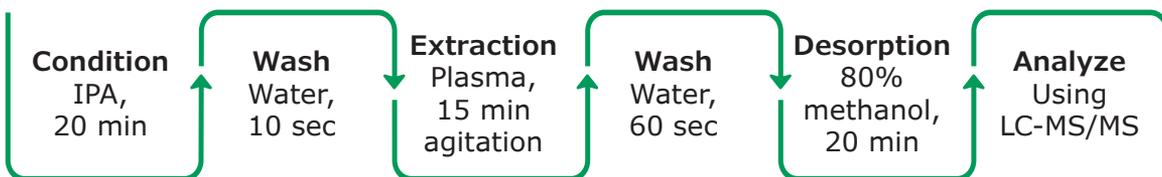
**Figure 1.** Overview of the steps for the Supel™ BioSPME 96-Pin device determination of free fraction of drug in human plasma.
