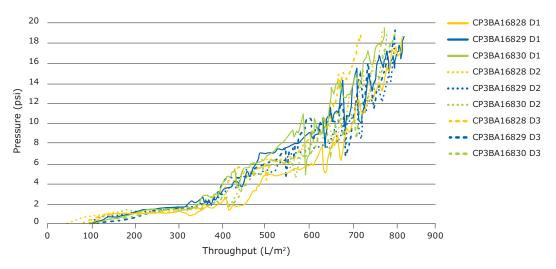
Figure 3. Lot-to-Lot Variability for Clarisolve® 40MS Depth Filters
