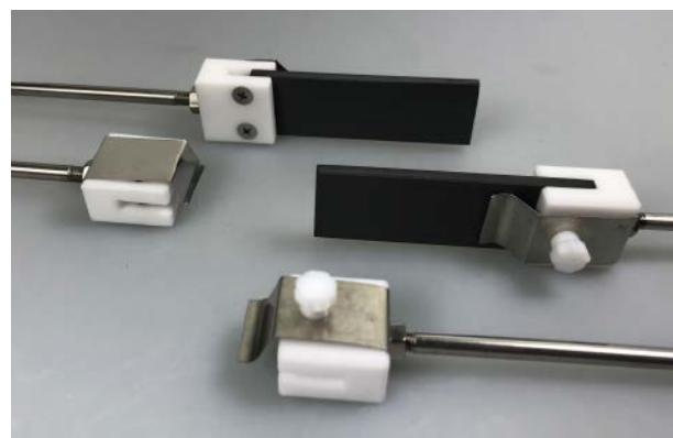
Figure 14. Electrode Holders for Mechanically Sensitive Electrode Materials. From Front to Back: Teflon® Electrode Holder with Stainless-Steel Spring Leaf for Facilitating Electrical Conductivity. The Leaf Is Fixed to the Electrode Holder with a Teflon® Screw. Side View of the Electrode Holder with a BDD Electrode Attached. Second Version of Teflon® Electrode Holder with Stainless-Steel Spring Leaf. Backside View of the Electrode Holder with Stainless-Steel Screws to Hold the Mounted BDD Electrode in Place.
