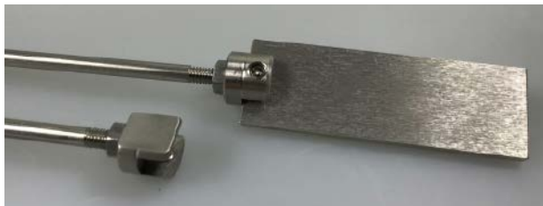
Figure 12. Standard Stainless-Steel Electrode Holder for Solid Electrode Materials. Front: View of the Flattened Side of the Electrode Holder. Back: Rear Side of the Electrode Holder with Screw and Mounted Electrode.
