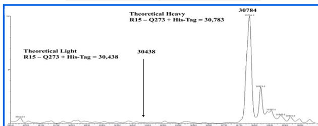
**Figure 2.** The intact mass of SIL-APOA1 was measured by SEC-MS using a 2 mm X 30 cm SEC TOSOH Bioscience (# 21485) column using 45% ACN 0.1% FA buffer. The MS data was collected on a Q-TOF Premier (Waters) and deconvoluted using MaxEnt1. The intact mass was found to be 30784Da, 32 ppm different from the theoretical value. No lock mass was used for the analysis.
