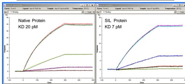
**Figure 4.** Binding curves for SIL-APOA1 and APOA1 isolated from sera (Academy Bio Medical #11P-101) with a goat polyclonal AB (R&D Systems AF3664). Data from a Biacore T100 (GE). There is very little difference between the binding of the native protein and the SIL protein. The difference in the KD measurements are due to the time for dissociation not being long enough to have an accurate measurement of  $K_d$ .
